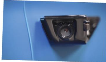
Camera monitoring system - camera
