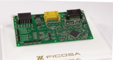
Battery management system
